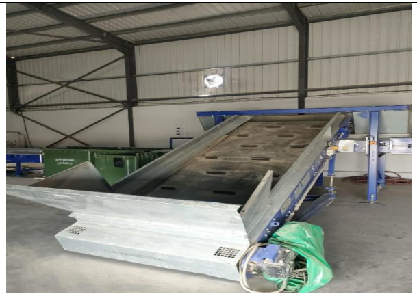
Figure 11 Sorting belt for mixed waste
